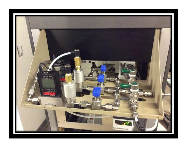
The Gas Delivery System for the Hitachi H-9500 E-TEM is designed to delivery up to 2 process gasses controlled in parallel and one evaporation liquid source. It has dry pump rough vacuum and built in nitrogen purge for fast process gas switching.
