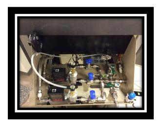
2) Verify that the evacuation valve is open and the pressure is below 7e-2 Pa. This is measured on the Varian gauge controller "AUX1".
