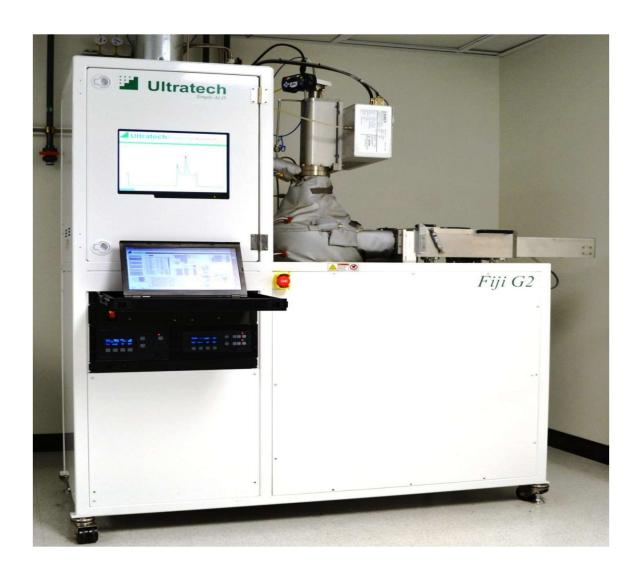
The Ultratech Fiji G2 is a modular, high-vacuum system accommodating multiple deposition modes using flexible system architecture and multiple configurations of precursors and plasma gases. The standard configuration of the Fiji G2 enables deposition of a wide range of materials including oxides, nitrides, and metals.
