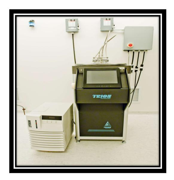
The Trion PECVD system has four process gases for deposition of films such as silicon dioxide, silicon nitride and poly-silicon. The system is controlled by a user-friendly touch screen computer system.
