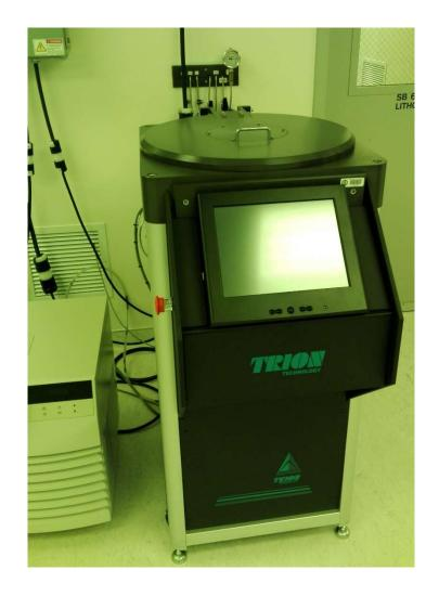
The Phantom III RIE system is designed to supply research laboratories with state-of-the-art-plasma etch capability for single wafers and small samples. Our RIE system has four process gases for etching a variety of materials. It can also be used for stripping photo-resists and other organic materials. The system is controlled by a user-friendly touch screen computer system.
