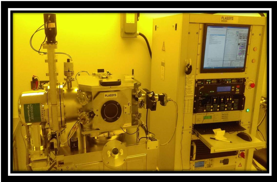
The model MEB 550-S provides thin film coating and Argon ION etching. Our system is equipped with 6 kW, 8-15cc pocket e-Gun, thickness monitoring, sample heater, and direct temperature monitoring. A variety of evaporation source materials are available. The system has an ultimate vacuum on the order of  $1.1 \times 10^{-8}$  mbar.
