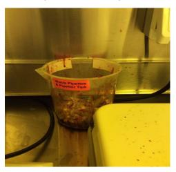
Waste pieces, broken samples or with lithography chemicals should be placed in marked beaker on hood's work surface.
