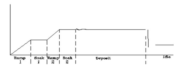
Phases of a Process Courtesy of Inficon
