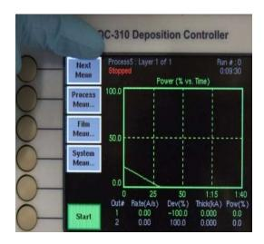
As soon as the Shutter delay is satisfied, the system will advance to the Deposit Phase, open the substrate shutter, zero the accumulated thickness and start depositing the Layer. Upon achieving a thickness set-point, the power will ramp down to 0% over a span of 30 seconds and the process will end. Allow 15 minutes for the source to cool and than press the vent button. Remove your sample, reinstall the sample holder and pump the system back down.
